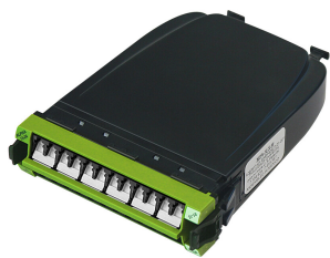
G2 LL Multimode OM5 MPO 12 distribution module, 24 LC to 2x12f MPO's pinned, internal shutters
