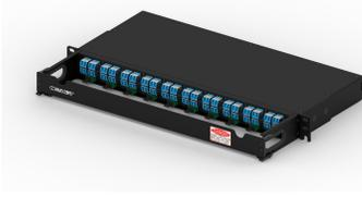
1RU patch panel which interfaces with QSFP ports to easily break them out in LC connections. The MPO and LC ports are both front facing for easy mapping and patching. 10 singlemode MPO-8 and 40 duplex shuttered LC ports, Method A
