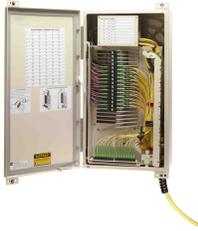
Enhanced Mini FDH, 72F loaded pole/wall mounted cabinet, SC/APC, preloaded w/ 1x 1:32 PNP splitter, I/O Dielectric Ribbon Cable, 100ft stubs using a 1x72F distribution cable assembly and a 1x12F feeder
