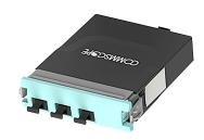
G2 ULL 1x3 Multimode OM4 Conversion Module, (1) MPO-24 unpinned ports rear, (3) MPO-8 pinned front
