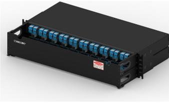
2RU patch panel which interfaces with MPO-8 ports including QSFP to easily break them out into LC connections. The MPO and shuttered LC ports are both front facing for easy mapping and patching. 20 singlemode MPO-8 and 80 duplex LC ports, Enhanced Method
