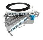
MFPS Fiber Optic panel, 2RU, 96 fibers/RU, pre-cabled I/O LSZH, 20m, front patch cords orientation to the right, 96 SC/UPC, grade C
