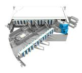
MFPS Fiber Optic panel, 2RU, 48 fibers/RU, splice/patch, SMOUV/front patch cords orientation to the right, 96 SC/UPC, grade C
