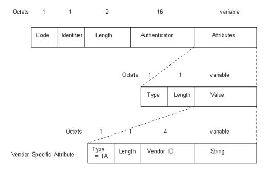
Figure 1 - RADIUS Packet Structure
