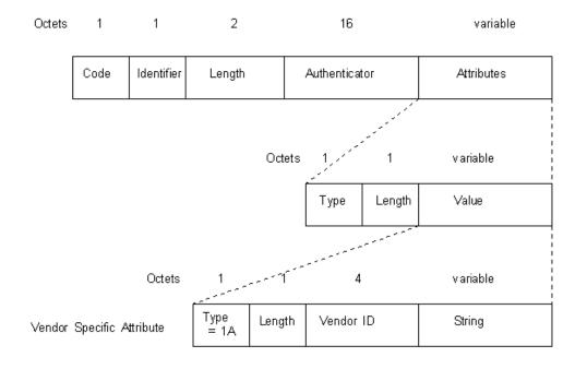
Figure 4 - RADIUS Packet Structure
