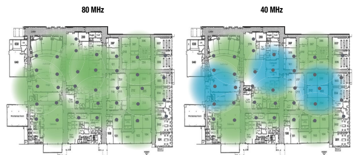
Figure 2: Spectrum Reuse with 40 and 80 MHz Channels
