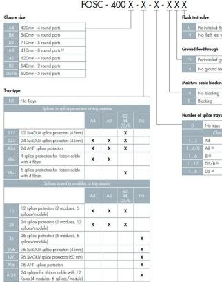
V Pre-installed flash test valve N No flash test valve Ground feedthrough © Pre-installed ground feedthrough N No ground feedthrough
