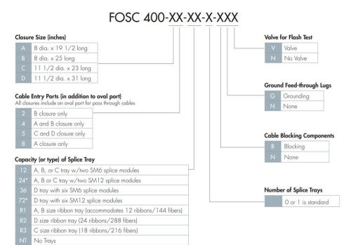
\*Note: SMOUV (1120-01-US) splice protection sleeves should be used with SM12 splice modules.
