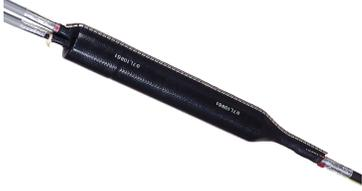
VCKT Vault Copper Closure, unpressurized, heat shrink, 740 mm joint length, 9 MDF cable outlets
