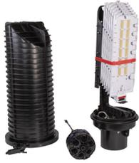
FOSC® 450 D6 Fiber Optic Splice Closure, Gel Cable sealing, three pre-installed 72-splice trays, 6 cable attach., six ground feedthrough lugs, with test valve
