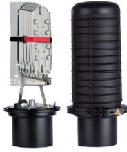
FOSC® 450 BS Fiber Optic Splice Closure, Gel Cable sealing, one pre-installed 24-splice tray, 6 cable attachments, with test valve
