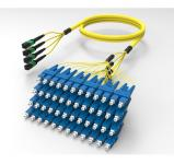
Singlemode MPO (Pinned) to SC/UPC, InstaPATCH® 360 Ruggedized Fanout Cable, 48-Fiber, Low Smoke Zero Halogen B2ca
