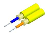
Fiber Indoor Cable, TeraSPEED® 1.6mm Low Smoke Zero Halogen Riser, 2-fiber Zipcord, Singlemode G.652.D and G.657.A1, Feet jacket marking, Yellow jacket color, Eca Flame Rating
