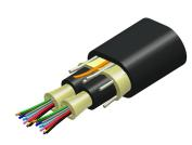
Fiber Indoor/Outdoor cable, LazrSPEED®, Low Smoke Zero Halogen Riser MPO Trunk Cable, 24 fiber with 12 fiber subunits, Gel-free, Multimode OM4, Feet jacket marking, Black jacket color, Dca flame rating
