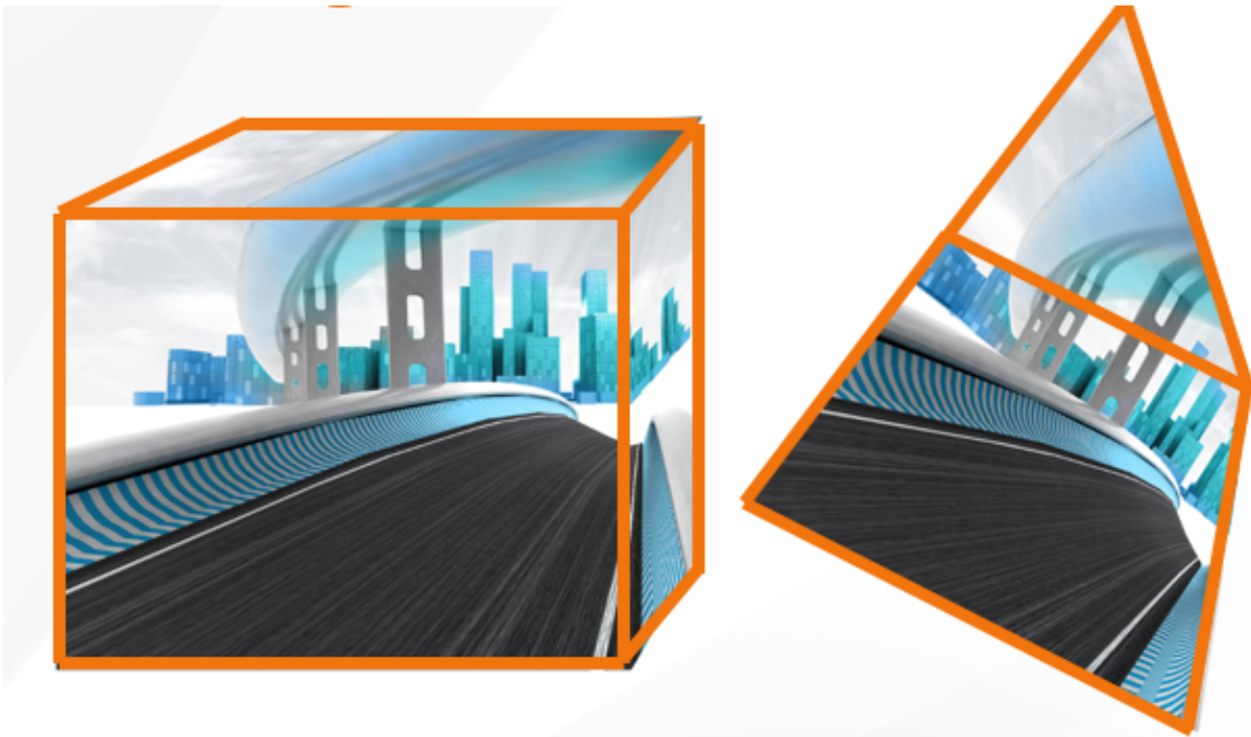
Figure 5 - Cube and Pyramidal Mapping of 360 Degree Scenes
