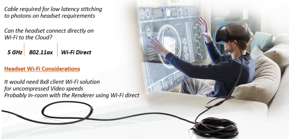
Figure 16 - Wi-Fi and VR HMD - Video Decoding Latency Prevents Its Use
