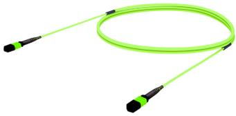
OM5 MPO (Unpinned) to MPO (Unpinned), InstaPATCH® 360 Array Cord, 12-Fiber, Low Smoke Zero Halogen
