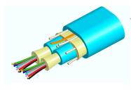
Fiber indoor cable, LazrSPEED®, Low Smoke Zero Halogen Riser MPO Trunk, 24 fibers, 12 fiber subunits, Multimode OM4, Gel-free, Feet jacket marking, Aqua jacket color, B2ca Flame rating
