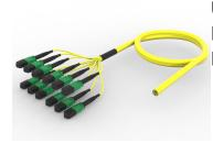
Ultra Low Loss (ULL) Singlemode, MPO12 Unpinned to Unconnectorized, Fiber Trunk Cable Assembly, 144-Fiber, Rollable Ribbon Central Tube, Plenum
