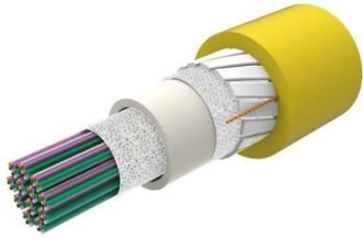
Fiber indoor/outdoor cable, All-Dielectric, LSZH, Riser-Rated, Gel-Free, Central Tube Rollable Ribbon, 144 fiber, Singlemode G.657.A2/B2, Feet jacket marking, Yellow jacket color, Cca flame rating
