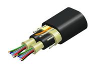
Fiber Indoor/Outdoor cable, TeraSPEED® Low Smoke Zero Halogen Riser MPO Trunk, 24 fiber with 12 fiber subunits, Gel-free, Singlemode G. 657.A2/B2, Feet jacket marking, Black jacket color, Dca flame rating
