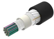
Fiber indoor/outdoor cable, All-Dielectric, LSZH Riser-Rated, Gel-Free, Central Tube Rollable Ribbon, 288 fiber, Singlemode G.657.A2/B2, Feet jacket marking, Black jacket color, Cca flame rating
