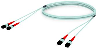
Ultra Low Loss (ULL) OM4 MPO24 (Pinned) to MP/24 (Pinned), Fiber Trunk Cable Assembly, 48-Fiber, Low Smoke Zero Halogen (LSZH)
