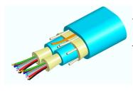
Fiber indoor cable, LazrSPEED®, Low Smoke Zero Halogen Riser MPO Trunk, 24 fiber with 12 fiber subunits, Gel-free, Multimode OM4, Feet jacket marking, Aqua jacket color, Dca flame rating
