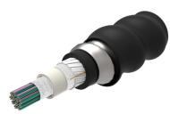
Fiber indoor/outdoor cable, Interlocking Armored, LSZH Riser-Rated, Gel-Free, Central Tube Rollable Ribbon, 864 fiber, Singlemode G.657.A2/B2, Feet jacket marking, Black jacket color, B2ca flame rating
