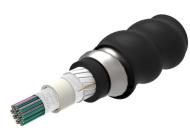
Fiber indoor/outdoor cable, Interlocking Armored, LSZH Riser-Rated, Gel-Free, Central Tube Rollable Ribbon, 288 fiber, Singlemode G.657.A2/B2, Feet jacket marking, Black jacket color, B2ca flame rating
