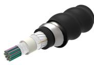
Fiber indoor/outdoor cable, Interlocking Armored, LSZH Riser-Rated, 144 fiber, Gel-Free, Central Tube Rollable Ribbon, Singlemode G.657.A2/B2, Feet jacket marking, Black jacket color, B2ca flame rating
