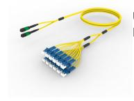
Ultra Low Loss ULL TeraSPEED® MPO(Pinned) to LC/APC G B Ruggedized fanout Cable, 24-Fiber, Plenum, 12 fiber PmP 2.0 mm Dca
