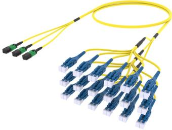
Ultra Low Loss ULL TeraSPEED® MPO(Pinned) to LC/UPC Uniboot Ruggedized fanout Cable, 36-Fiber, Plenum, 12 fiber PmP 2.0 mm Dca
