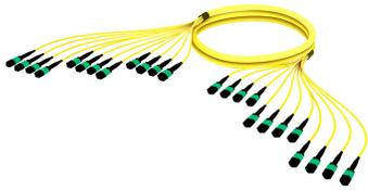
Singlemode MPO12 (Unpinned) to MPO12 (Unpinned), Fiber Trunk Cable Assembly, 144-Fiber, B2ca, Method A, Low Smoke Zero Halogen
