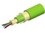
Fiber indoor cable, LazrSPEED® Low Smoke Zero Halogen Riser MPO Trunk with 2.0mm Subunits, 12 fiber, Multimode OM5, Gel-free, Feet jacket marking, Lime green jacket color, Dca Flame rating
