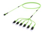
Ultra Low Loss ULL LazrSPEED® 550 OM5 MPO(Pinned) to LC/UPC Uniboot Ruggedized fanout Cable, 12-Fiber, LSZH, 12 fiber PmP 2.0 mm Dca
