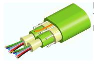
Fiber indoor cable, LazrSPEED® Low Smoke Zero Halogen Riser MPO Trunk, 24 fiber with 12 fiber 2.0mm subunits, Gel-free, Multimode OM5, Feet jacket marking, Lime green jacket color
