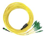
Multi Distribution Break Out Cable Singlemode MPO/8 equipment unpinned to SC/APC, 8 fibers, LSZH, 30 meters
