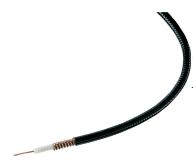
Heat Treated FSJ1RK-50B, HELIAX® Superflexible Foam Coaxial Cable, corrugated copper, 1/4 in, black non-halogenated, fire retardant polyolefin jacket
