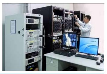
Lightning protection surge testing is a part of EMC compliance testing refer from IEC61000-4-5 and UL1449 standard, typically equipment output with 1.2µs/50µs or 8µs /20µs pulse surge generator and max capability with 20KV (10KA). Testing typically focused on RET, AISG/bias tee/AILP board and other electrical/active PCBA plus filters, in addition, some of RF port surge verification at different surge level is also required.
