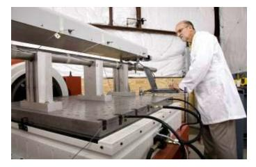
**UV weatherization testing** is done on radome and other polymer materials that may be exposed to sunlight following IEC 60068-2-5 and ETS 300 019-1-4 class 4.1E conditions
