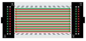
Figure 4: 100GBASE-SR10 full duplex operation on 20 fibers
