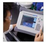
The International Electro-technical Commission (IEC) developed a series of five tests to measure PIM caused by dynamic factors such as flexing, tapping or pulling, duplicating the effects of adverse weather conditions at the top of a tower.
