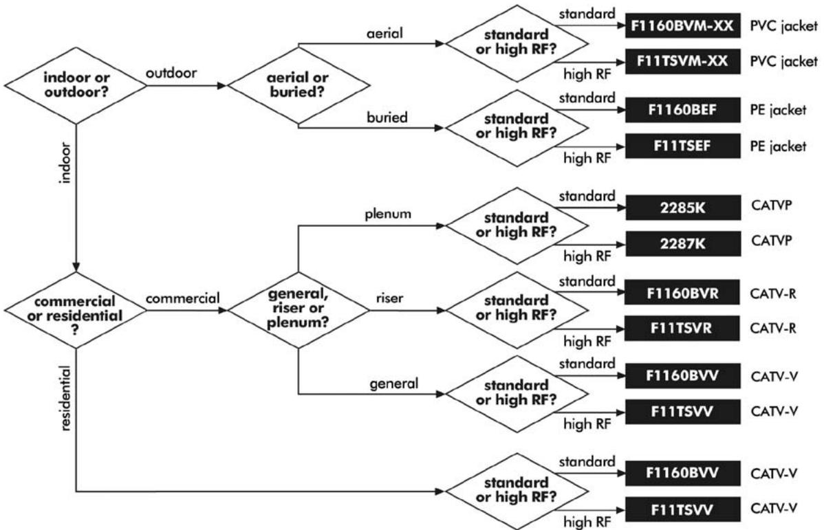
The XX in the part number should be filled with the code for the anti-corrosion agent you'd prefer as follows: **BW** for CommScope's dry BrightWire®, or **APD**® for the more traditional APD flooding compound. All nonplenum high RF cables are tri-shielded (foil/60 percent braid/foil); super-shield versions are available. Plenum cables are available only with super-shields.
