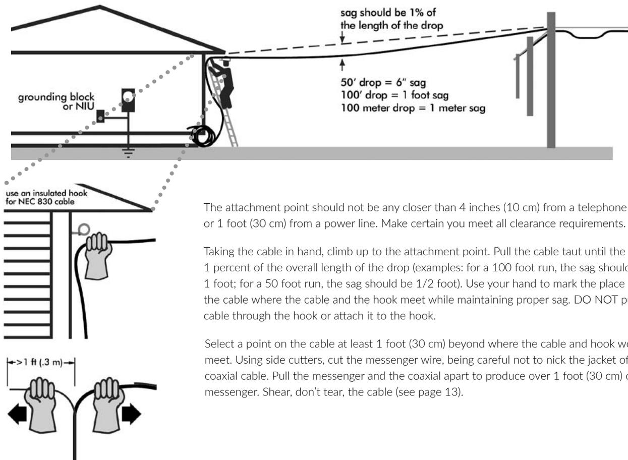
The attachment point should not be any closer than 4 inches (10 cm) from a telephone cable or 1 foot (30 cm) from a power line. Make certain you meet all clearance requirements.
