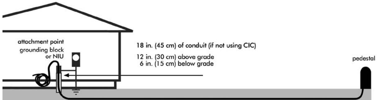
conduit to the wall with U-clamps so that 6 inches (15 cm) of cable is below grade and 12 inches (30 cm) is above grade. Seal the end of the conduit with either a waterproof expanding foam or with a duct cap.
