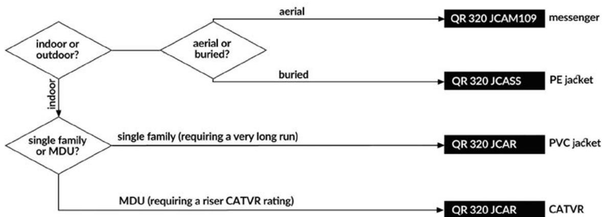
QR 320 cables have a unique welded aluminum strip shield for superior RF protection and a large center conductor for lower attenuation over longer distances. We recommend them for use in MDUs.
