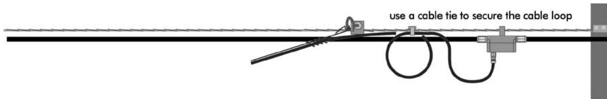
Store this cable by forming a loop of about 6 inches (15 cm) in diameter. Make sure the diameter of the loop is no smaller than 10 times the outer diameter of the cable. Use cable ties to form and secure the loop to the span.
