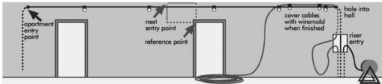
Use a stud finder to make sure you are drilling into a wall cavity. If possible, fish the cable down to the outlet location. Review page 22 (residential interior cabling) for details.
