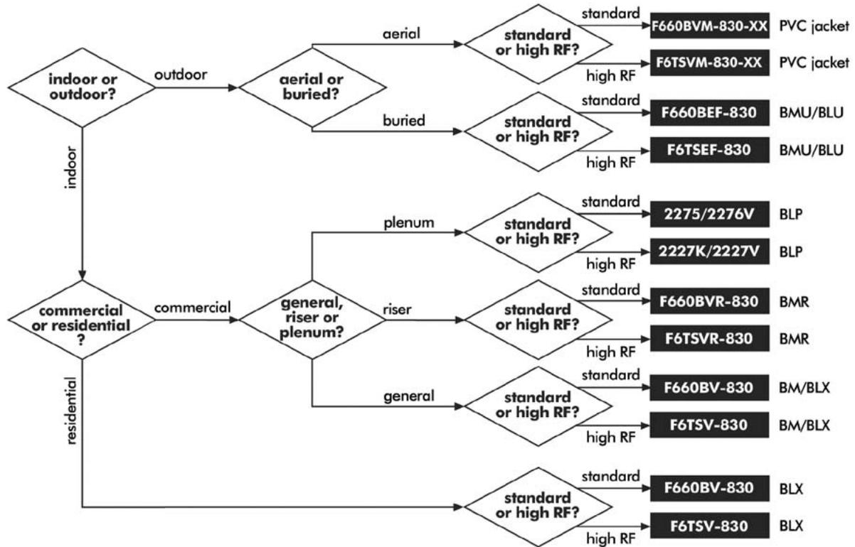
**BW** for CommScope's dry BrightWire®, or **APD**® for the more traditional APD flooding compound. All nonplenum high RF cables are tri-shielded (foil/60 percent braid/foil); super-shield versions are available. Plenum cables are available only with super-shields. A 90 percent braid is available for 2276K.
