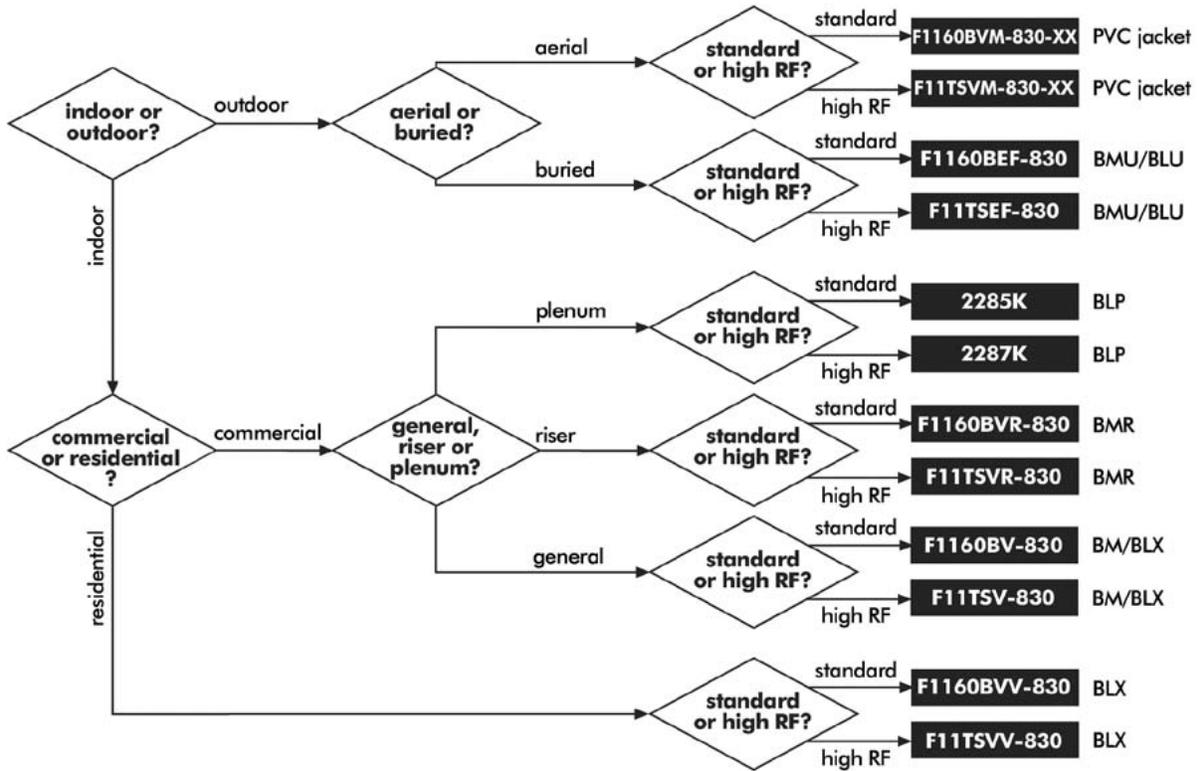
**BW** for CommScope's dry BrightWire®, or **APD**® for the more traditional APD flooding compound. All nonplenum high RF cables are tri-shielded (foil/60 percent braid/foil); super-shield versions are available. Plenum cables are available only with super-shields.
