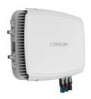
Carrier Access Point with 4-Band Support for Low Power CEL 900, DCS 1800, IMT 2100, and IMT 2600 Applications, Copper Fed, External DC Powered, with Fan Kit
