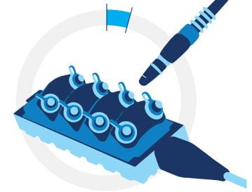
Use of pre-terminated connectors eliminates splicing,
