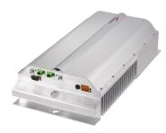
ION®-B Series High Power Remote Unit for LMR 700, LMR 800, Cellular 850, LMR 900, AWS, and PCS 1900
