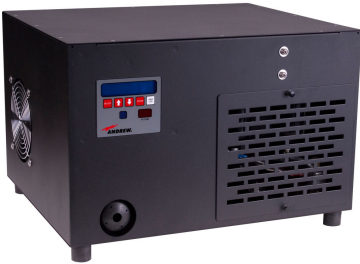
DryLine® Dehydrator, Low-pressure membrane, 2.0–5.0 psig, with discrete alarm, 240 Vac, 50/60 Hz
