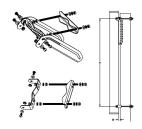
Adjustable Tilt Pipe Mounting Kit for 2.0"-4.5" (50-115mm) OD round members for panel antennas. Includes 2 clamp sets.
