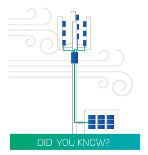
**FTTA hybrid direct trunk cables** can support up to *9 remote radio units,* minimizing space requirements.
