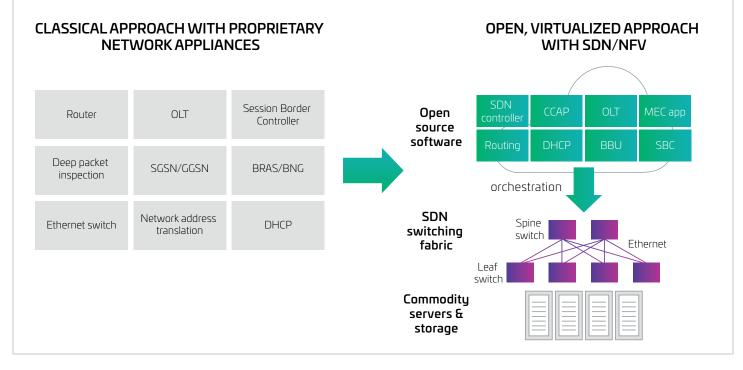
Figure 2: From proprietary appliances to an open, virtualized environment
