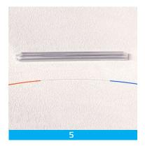
Spliced fibers and protective sleeve (SMOUV)
