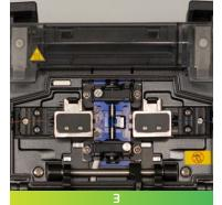
Fibers are joined in a fusion splicer
