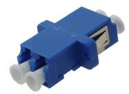
Fiber Optic Duplex Adapter, Singlemode, LC/UPC, ceramic sleeve, blue, flanged with metal clip, white dustcaps
